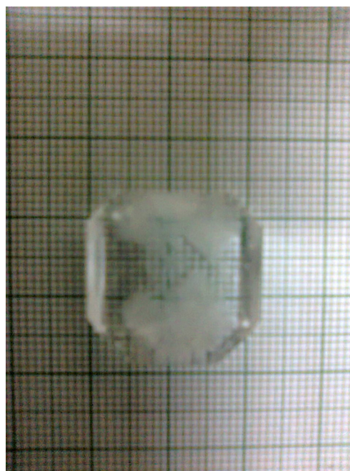
Fig. 1. Photographs of as grown single crystal of LAAD from the suspended seed.
