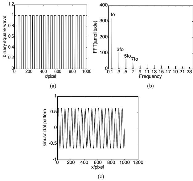
**Fig. 1.** Theory of sinusoidal fringe generation by defocusing a binary square wave: (a) the binary square wave, (b) the odd harmonics of the binary square wave, and (c) the ideal sinusoidal fringe.
