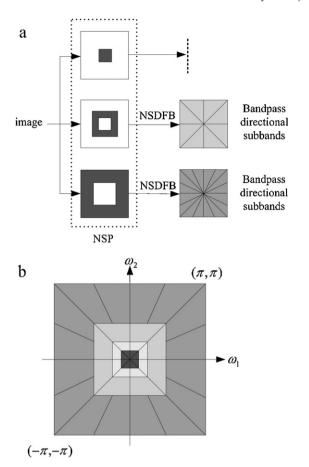
**Fig. 1.** The nonsubsampled contourlet transform. (a) Nonsubsampled filter bank structure that implements the NSCT. (b) The idealized frequency partitioning obtained with the proposed structure.
