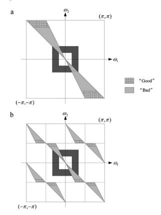
**Fig. 2.** The need for upsampling in the NSCT. (a) With no upsampling, the highpass at higher scales will be filtered by the portion of the directional filter that has "bad" response. (b) Upsampling ensures that filtering is done in the "good" region.
