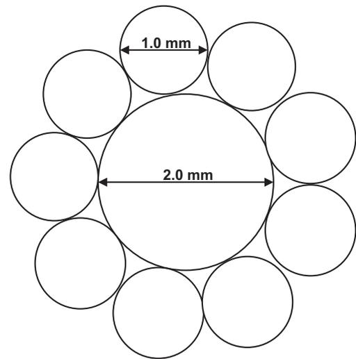
**Fig. 2.** Schematic showing the arrangement of the air-cooled fiber-optic probe excitation and collection fibers. The center 2000 μm diameter fiber is used for delivering the 266 nm pulsed laser beam to the phosphor coated target and the surrounding nine 1000 μm diameter fibers are used for collecting the emitted fluorescence radiation from the engine part.
