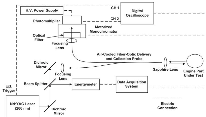
**Fig. 1.** Schematic showing the Nd:YAG (operating at 266 nm) laser-based system incorporating air-cooled fiber-optic probe for high-temperature 1-D intensity and decay lifetime thermographic phosphor fluorescence measurements.
