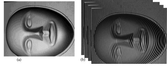
Fig. 1. Tested object and deformed fringe. (a) Tested mask and (b) four-step phase-shifting sinusoidal patterns are projected on the tested mask
