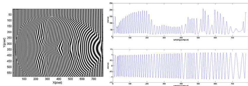
Fig. 2. (a) Deformed pattern after normalization and (b) comparison of the same cross section ( $j = 300$ ) before and after normalization.
