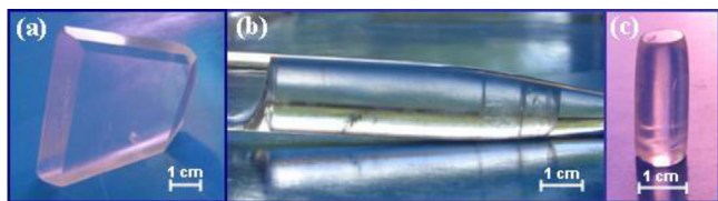
Fig. 1. (a) Conventionally grown LAHBr single crystal (b) Unidirectionally (001 plane) grown LAHBr single crystal with ampoule and (c) cut and polished LAHBr single crystal.
