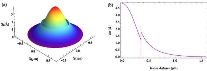
Fig. 1. Power profile for the air-clad single mode silica nanowire at 1.55  $\mu\text{m}$  wavelength.
