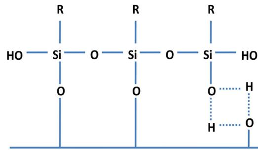
Fig. 2. Bond formation in silation process.
