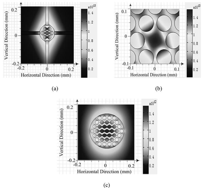
Fig. 2. (a) Near-field image of steering-wheel MOF air-hole cladding. (b) Near-field image of the traditional solid-core PCF. (c) Near-field image of the traditional porous optical fiber.
