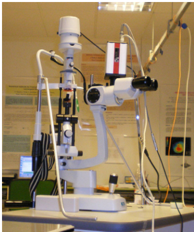
Fig. 1. Slit-lamp and digital video camera used to capture the images of frontal corneal.
