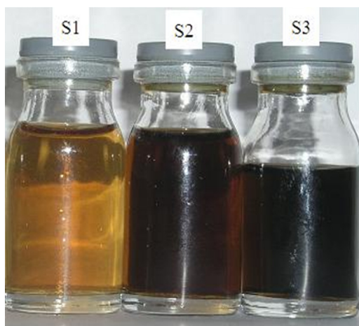
Fig. 1. Produced Ag nanoparticles with laser ablation in acetone.
