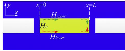
Fig. 3. Schematic of SPP described by the magnetic field propagating oppositely at interfaces.
