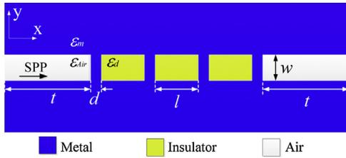
Fig. 1. Schematic of the SPP filter with triple periodic cascade cavities.
