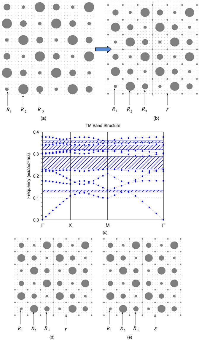
**Fig. 1.** Physical model of symmetrically perturbed photonic crystal. (a) Structure of photonic crystal with the radius of its rods distributed according to proportion as  $R_1 : R_2 : R_3 = 0.1a : 0.3a : 0.2a$ ; (b) structure of intact symmetrically perturbed photonic crystal; (c) Band diagrams; (d) first optimization: adjusting the radius of perturbative dielectric rods; (e) second optimization: adjusting the dielectric constant of perturbative dielectric rods.
