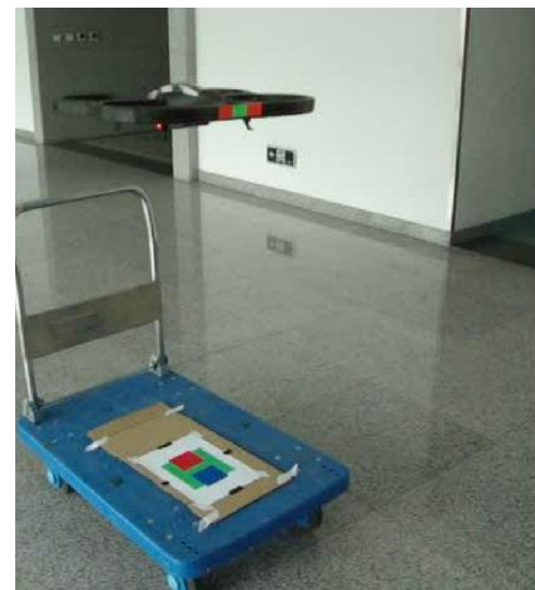
Fig. 2. Pushcart carrier with the green helipad and two color rectangles. (For interpretation of the references to color in this figure legend, the reader is referred to the web version of the article.)
