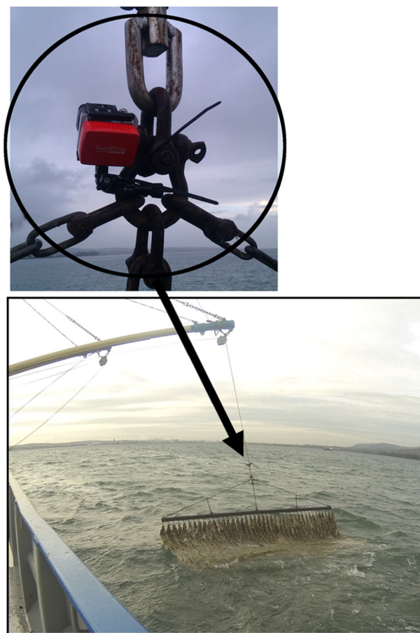
Fig. 1. GoPro™ camera on the starfish mop deployed from the starboard side of a mussel dredger in Belfast Lough.
