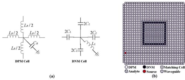
**Fig. 1.** Schematic structures of the simulation model. (a) Unit cells; (b) computational domain of the SWGM resonator.
