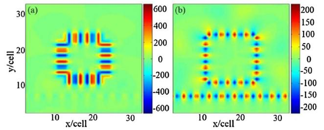
**Fig. 2.** Voltage distribution in the computational domain of the resonator. (a) With metamaterials; (b) without metamaterials.
