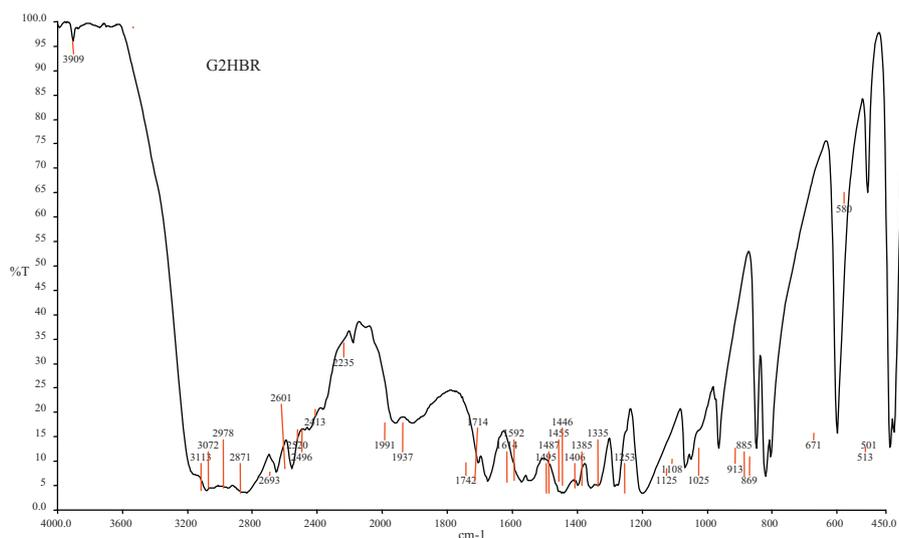
Fig. 2. FTIR spectrum for the BGHBR crystal.
