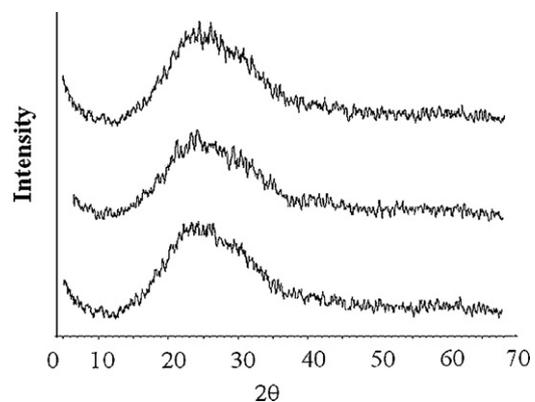
Fig. 2. XRD patterns of titanium/glass layers with different deposition angles.
