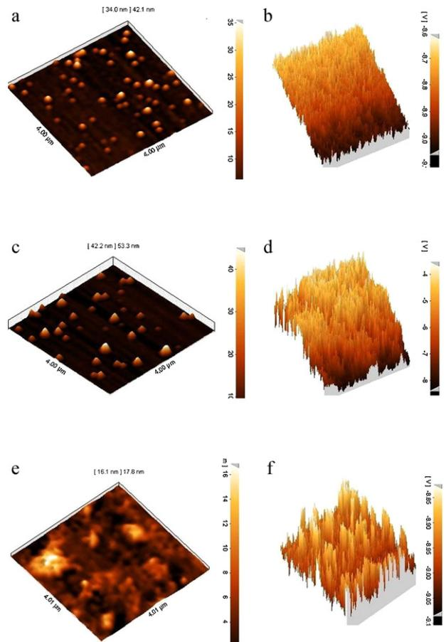
Fig. 1. AFM images of titanium/glass layers with different deposition angles.
