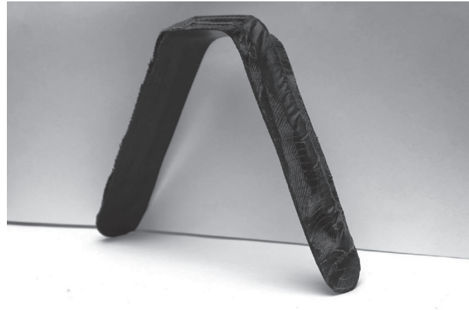
Figure 2. The U-shaped trapezoidal support shaft crafted from stainless steel rod laminated with stringed carbon fiber. Color version available online.
