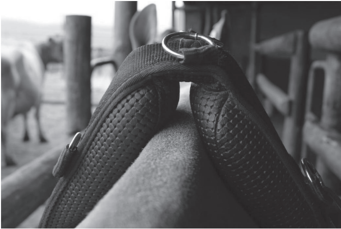
Figure 1. Harness body showing the perforated neoprene padding with built-in support shaft to ensure breathability and comfort to the trapezius area of the cow while acting as a platform for attachment of the gas collection vessel. Color version available online.
