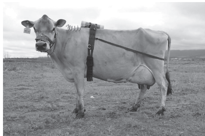
Figure 3. A Jersey cow equipped with a simple back-mounted harness for gas collection vessel attachment to facilitate the SF 6 tracer gas technique. Adjustable buckles and elastic band over the flank avoid dislodgment of the harness. Color version available online.
