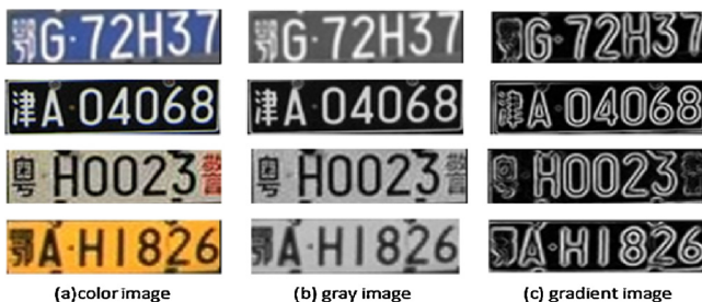
Fig. 2. Examples of color license plate image, gray image and gradient image.
