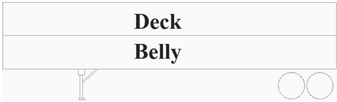
Figure 1. Internal straight deck livestock trailer schematic diagram displaying the separate compartments used to transport cattle.
