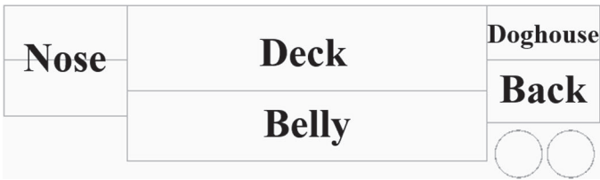
Figure 2. Internal potbelly livestock trailer schematic diagram displaying the separate compartments used to transport cattle.
