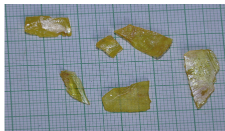
Fig. 3. Photograph of as grown crystal of SAN NLO crystal by slow evaporation method.
