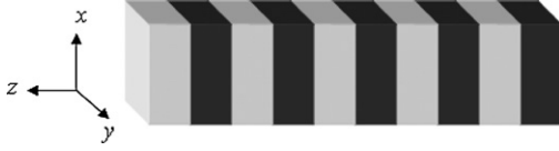
Fig. 1. Schematic of the PBG structure with a double-layer unit cell of anisotropic RHM and LHM.
