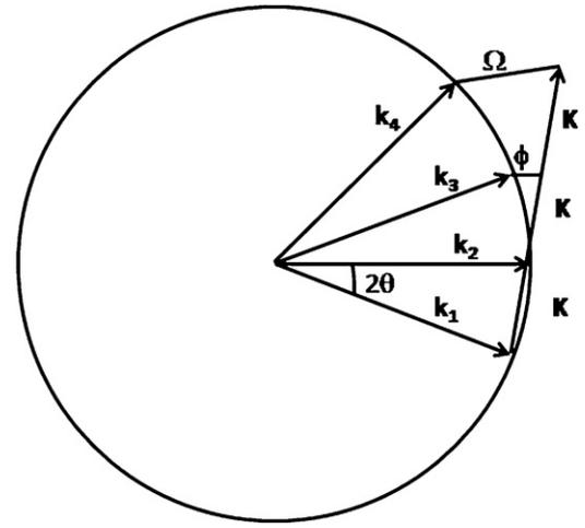
**Fig. 2.** Ewald sphere construction relating the interacting wave vectors and the grating vectors ( $k_1, k_2, k_3$  and  $k_4$  are the propagation vectors of the beams *A, B, C* and *D* respectively).
