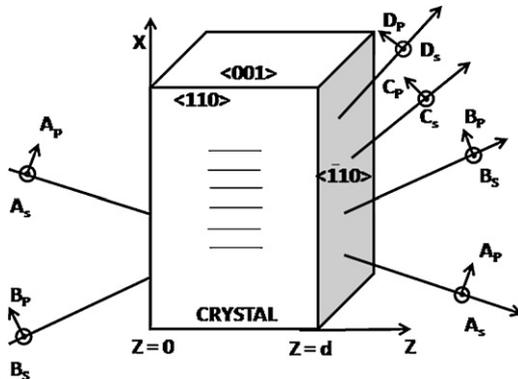
**Fig. 1.** Input beams and higher diffraction orders in two-wave mixing in transmission geometry (here *A* is the Pump Beam, *B* is the Signal Beam, *C* and *D* are the first and second higher-order diffracted beams).
