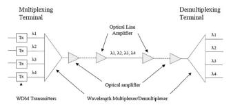
Fig. 1. A typical WDM link.
