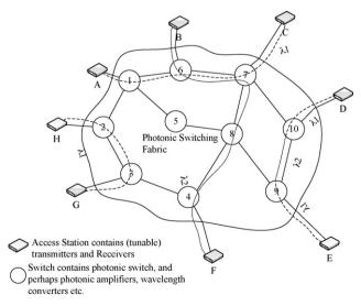
Fig. 2. Wavelength-routed WDM optical network.
