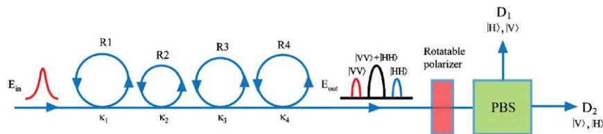
**Fig. 1.** A schematic of the design system. PCs: polarization controllers, Ds: detectors—Avalanche photo-detector and PBS: polarization beam splitter.
