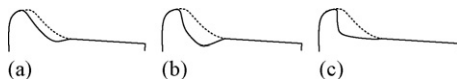
Fig. 2. Sketch diagram of different flange wearing. (a) Thin after wearing, (b) sharp after wearing and (c) orthogonal after wearing.
