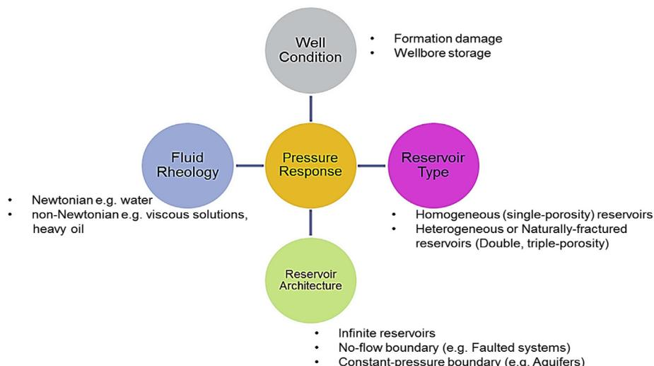
Fig. 1. Factors influencing pressure behavior of fluids flowing through porous rocks.
