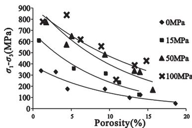
Fig. 2. Porosity versus peak stress at different confining pressures.
