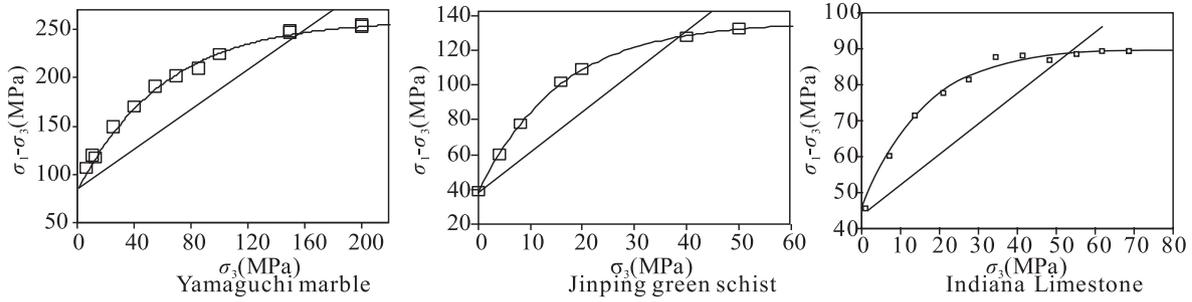
Fig. 1. Fitting curves of the strength and confining pressure for different rock types.
