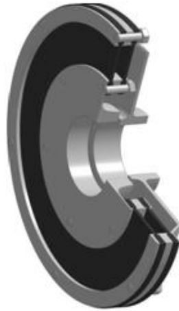
Fig. 1. Three-dimensional model of the rubber-cord flat coupling with two working elements
