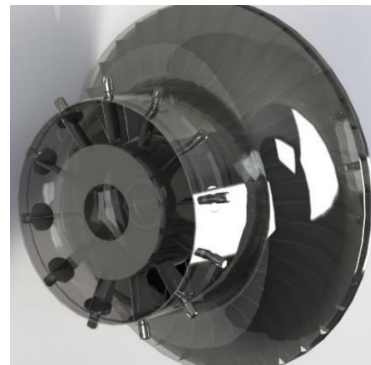
Fig. 2. 3D model of the impeller and inlet guide vane unit.
