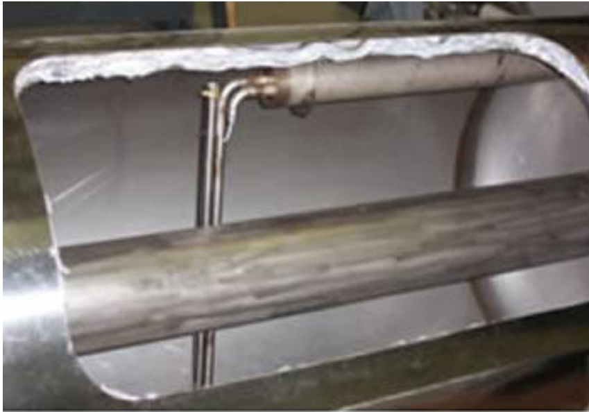
Fig. 1. The superinsulated cryogenic tank for LNG.
