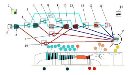
Fig. 1. Topological model of afterburning turbofan engine in SIM Dvig\_Otladka, where 1 – ambient conditions; 2 – input device; 3 – low pressure compressor; 4 – gases selection; 5 – high pressure compressor; 6 – gases selection 2; 7 – combustor chamber; 8 – air-to-air heat exchanger; 9 – power selection; 10 – power selection 2; 11 – gases selection 3; 12 – high pressure turbine; 13 – low pressure turbine; 14 – flow mixer; 15 – afterburner; 16 – jet nozzle; 17 – regulator; 18 – total result.
