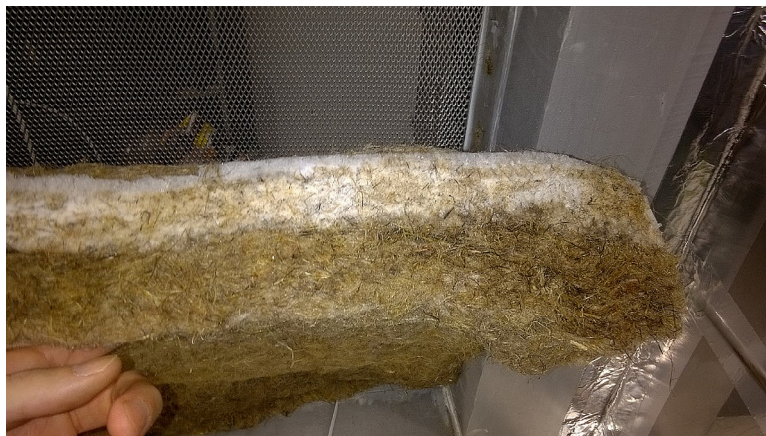
Fig. 1. Ice formation on a test sample caused by humid air penetration.
