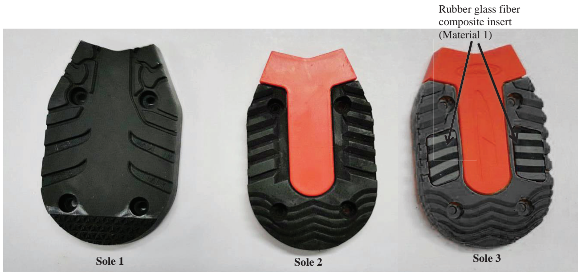
Figure 1. Soles used in the present study, indicating the zone of the rubber/fiber composite insert position in Sole 3.
