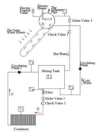
Fig. 1.Solar kang heating system
