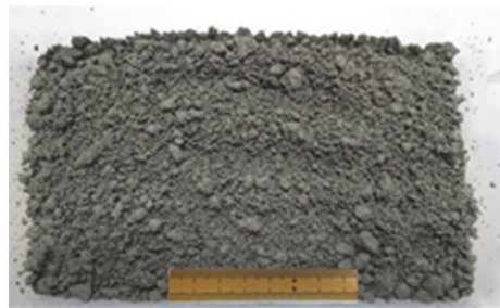
Photo 1: Granules produced by crumbling granulation
