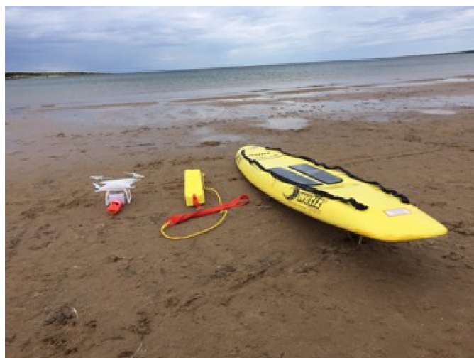
Figure 2. Rescue equipment from left to right: a drone equipped with an inflatable life buoy (intervention), a torpedo buoy for rescue swimming (control), and a rescue board for paddling.
