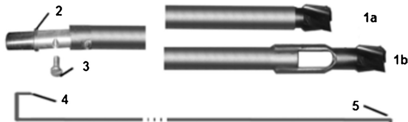
Fig. 2. (1–5) Schematic illustration of the borer and extractor components: 1a and b modifications of the tenon plug cutter, 2 adapter, 3 locking bolt, 4 handlebar, 5 cutting blade.
