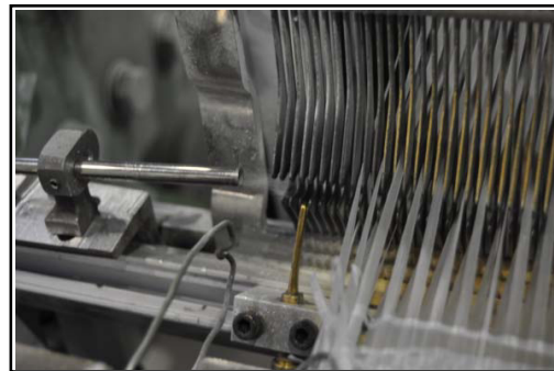
Fig. 2 Positions of the main nozzle and the sub nozzle.
