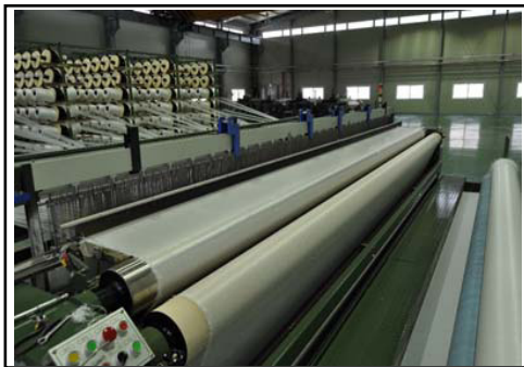
Fig. 1. The setup of air jet loom equipment.
