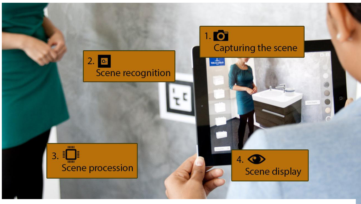
Fig. 1. Augmented reality display principle - V&B Augmented Reality App [11].
