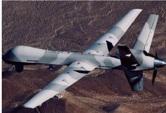
Fig.1 Propeller thrusting layout of Predator UAV
