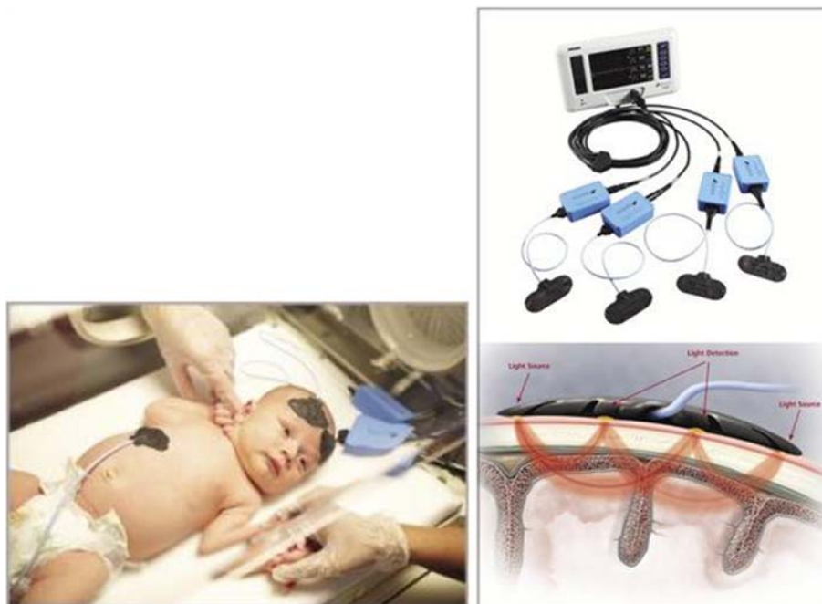
Fig. 1. Nonin Medical, Inc. (n.d.), Accurate, Portable Cerebral/Somatic Tissue Oximeters (rSO 2 ) . Retrieved from http://static-96-232-192-10.nycmny fios.verizon.net/ancp/0812/content/ANCP12_036a.html# . Permission from Nonin Medical, Inc., n.d. The EQUANOX™ Model 7600 Cerebral/Somatic Tissue Oximetry System is a NIRS-based monitoring device that noninvasively and continuously detects oxygen saturation status in brain and other tissues.
