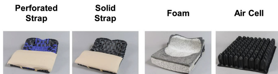
Fig. 1. Images of the four seating systems tested for microclimate characteristics including two strap-based seating systems, a foam-based and an air cell-based seating system.
