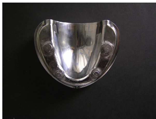
Fig. 1 CAD/CAM designed stainless steel die.
