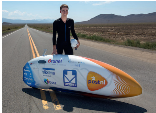
Figure 1. Velox3, recumbent fully faired bicycle, which holds the current World Human Powered Vehicle speed record for single rider vehicles at 133.78 km/h.
