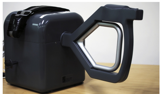
Fig. 1. A custom-made multifunctional hand strength measurement device.
