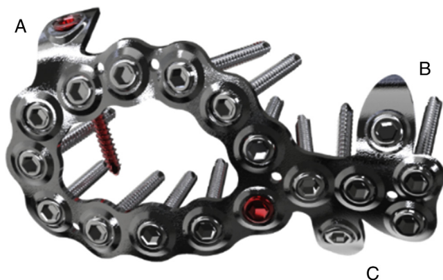
Fig. 1. The anatomic locking plate for calcaneus fractures. The left side of the plate is for the posterior calcaneus and the right is for the anterior calcaneus process. A indicates the Achilles fin, B, the sulcus calcaneus fin, and C, the plantar fin. The 2 red screws are designed for tongue-type fractures and sustentaculum tali, respectively.
