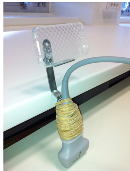
Fig. 1. Illustration of the iPhone attached to the ultrasound probe for the measurement of accelerations of the probe during catheter insertion.
