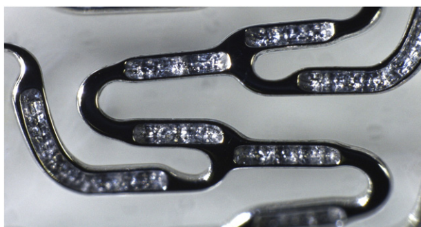
Fig. 1. Macroscopic picture of the abluminal reservoirs on the surface of the Cre8 stent, filled with an amphilimus formulation (obtained with permission of Moretti C. et al. [4]).
