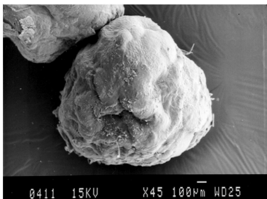
Fig. 1. Aerobic granular sludge by SEM (scanning electronic microscope) [3].
